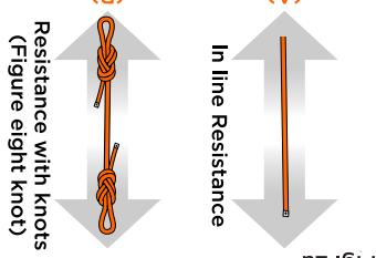
THICK-LINE 10.5: 21kN / 14kN
